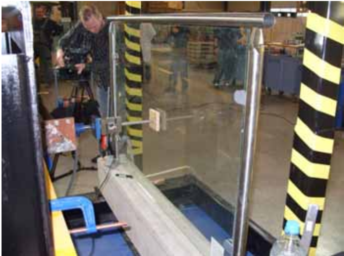
Photograph 3 Extra Strong system during point load test
