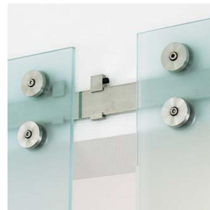
the fitting 700 is suitable for smaller systems and weights of the door leaf up to 60 kg. the special feature is the vertically mounted flat steel track and the small castor. particularly suitable for displaycases, cabinets, showers, all-glass systems, sliding shutters, media cabinets, etc. the polyamide surface allows a very quiet running. the supporting bar 50/6 is used for doors, for displaycases e.g. 30/6 is used to get a more airy appearance.
