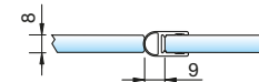
art. no. 8861KU0-8-2010 art. no. 8861KU0-8-2500 for 6 and 8 mm glass for a pendulum shower hinge
