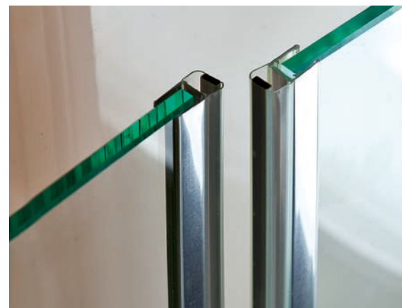
art. no. 8850KU7-8-2010 sealing profile for glass-glass 180° for 6 and 8 mm glass for a double- sided opening.
